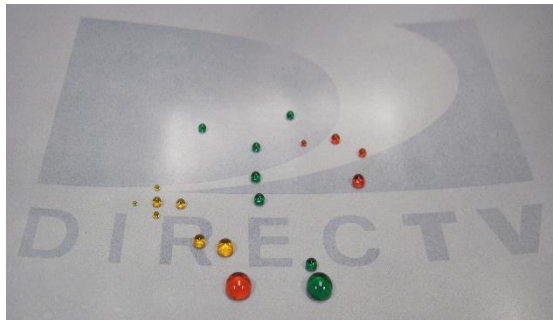
Colored water is repelled & forms beads on FluoroThane WT coated surface
