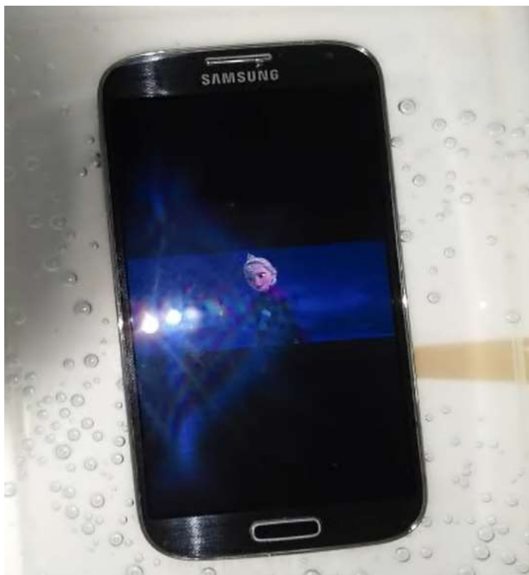
Figure 1. Smartphone coated with FluoroPel working under water passes IPX5 or IPX7 water resistance test
