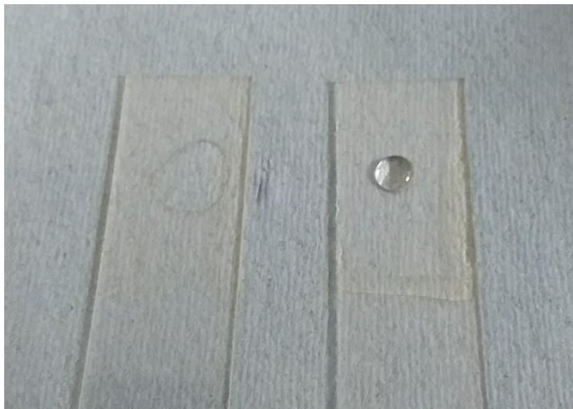
25 microliters of mineral oil on SR399 UV-curable coating compared to SR399 plus 2% FluorAcryl 7298
