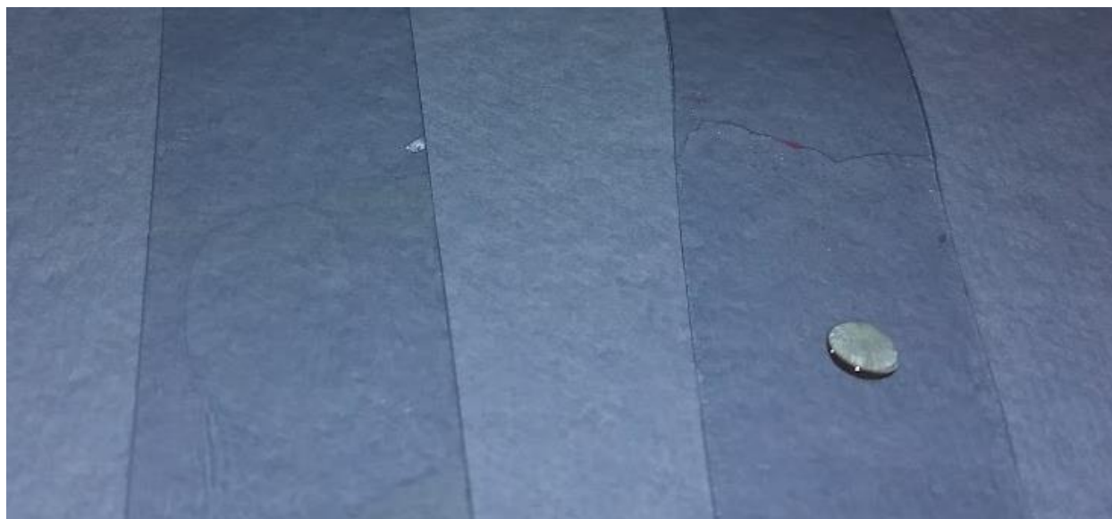
25 microliters of clover oil on a UV-cured film of CN9302 and SR351 (50:50) compared to CN9302 and SR351 (50:50) plus 2% FluorAcryl 7298
